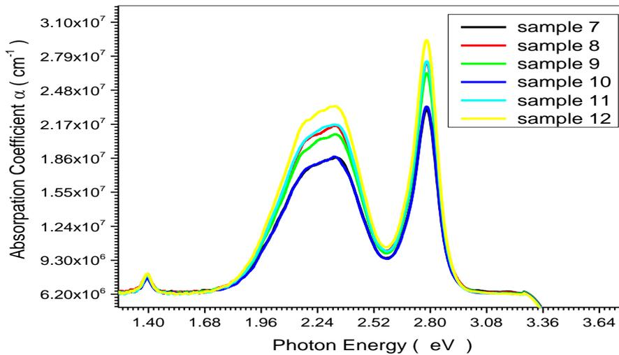
Figure (2.a.2) Absorption coefficient versus photon energy for all samples
